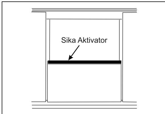
FIGURE 72 : SLIDING WINDOW - SIKa AKTIVATOR
