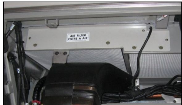
PASSENGERS AREA AIR FILTER REMOVAL
