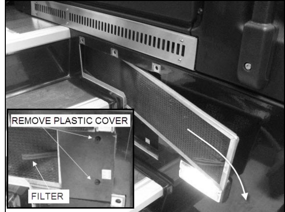
REMOVING DRIVER'S SECTION AIR FILTER
