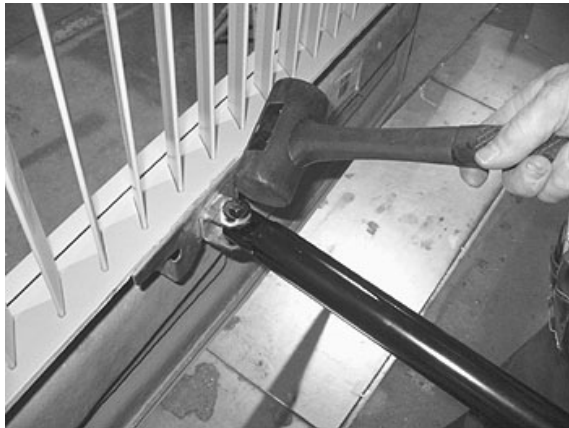
FIGURE 64: DOOR LATERAL ADJUSTMENT
