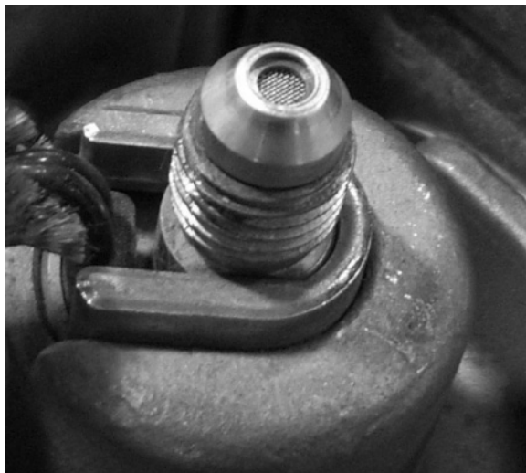
FIGURE 13 : AFTERTREATMENT FUEL INJECTOR INLET SCREEN
