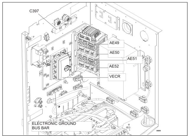
8. Before connecting the harness, locate the following components in the main electrical compartment
