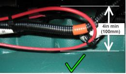
LTD is not a flexible harness. Avoid tight bends and kinks which could short circuit the LTD. Loops must hace a minimum radii of 4 inches (100 mm)
