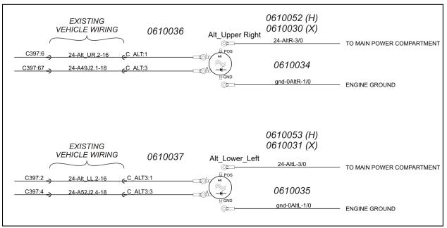
FIGURE 1: ALTERNATOR CONNECTIONS W/ HARNESS NUMBERS
