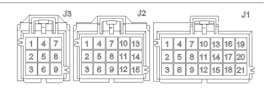
**FIGURE 4: IOEB PINOUT**
