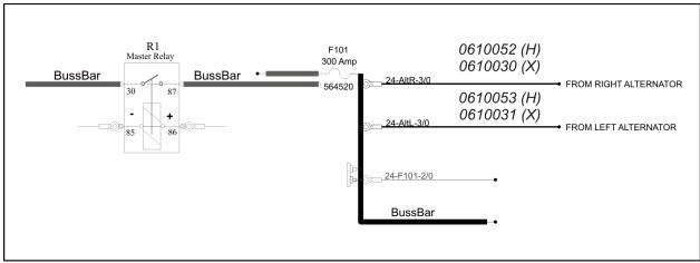
FIGURE 2: POWER CABLE CONNECTIONS IN MAIN POWER COMPARTMENT
