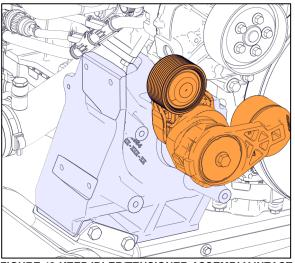
FIGURE 49: IDLER / TENSIONER ASSEMBLY MOUNTING SCREWS
