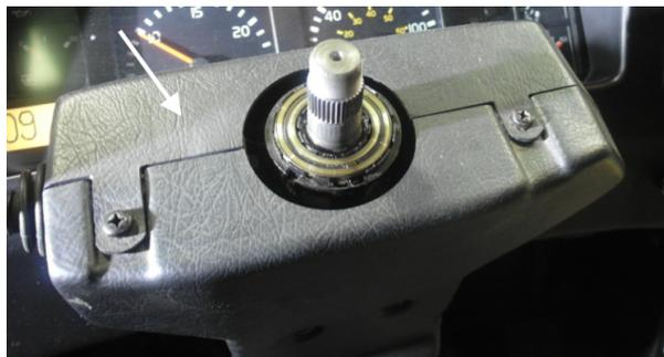
7. Install adapter ring **160004** to the new steering wheel **661171**.
