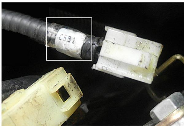
4. Route & connect new harness extension **0610188** from the steering column to the lateral control panel.
