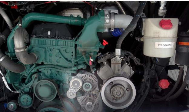
FIGURE 2: BOSCH ALTERNATORS ON ENGINE
