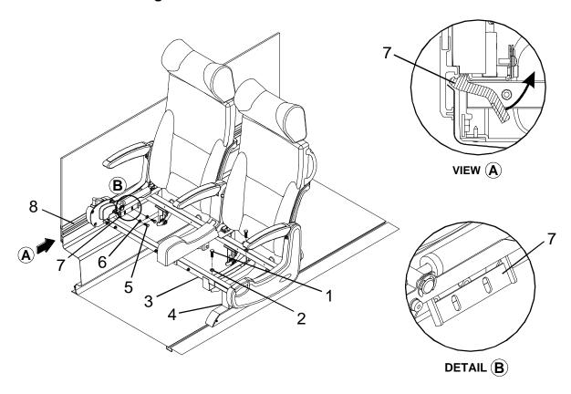
Figure 2-1 Two-Passenger Seat Frame Removal
