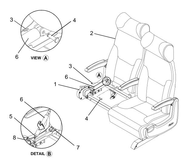
Figure 2-14 Reclining Gas Cylinder Replacement
