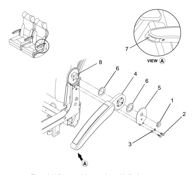
Figure 2-16 Downward Armrest Assembly Replacement
