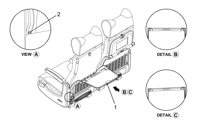
Figure 2-32 Tray Table Slant Adjustment
