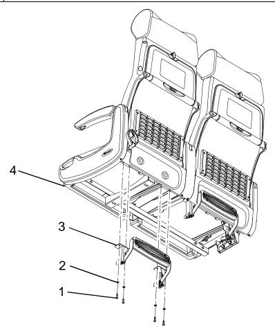
**Figure 2-21 Footrest Assembly Replacement**
