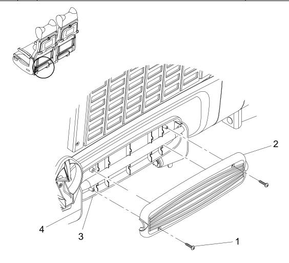
Figure 2-22 Footrest Plastic Cap Replacement
