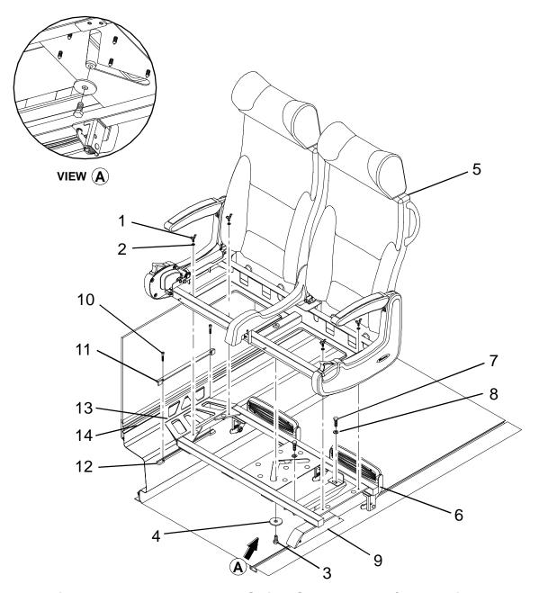
Figure 2-3 Two-Passenger Swivel Seat Removal / Installation
