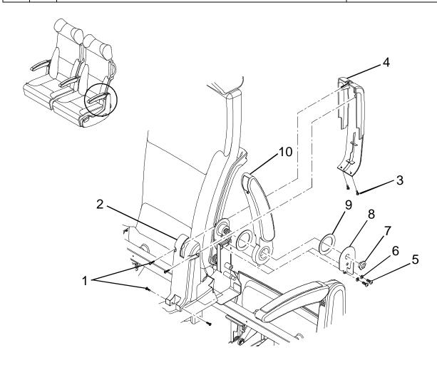
**Figure 2-17 Center Upward Armrest Assembly Replacement**
