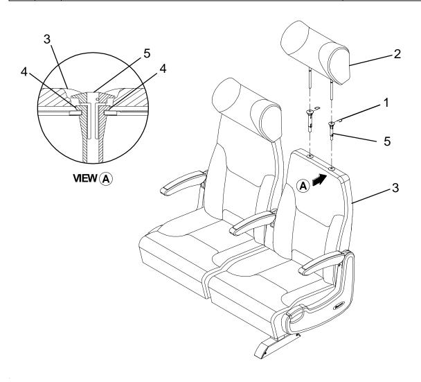
Figure 2-8 Headrest and Sliding Guide Replacement
