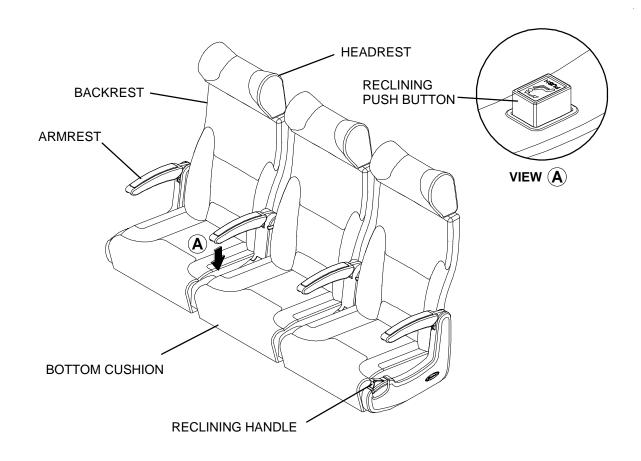
Figure 1-3 Three-Passenger Bench Seat
