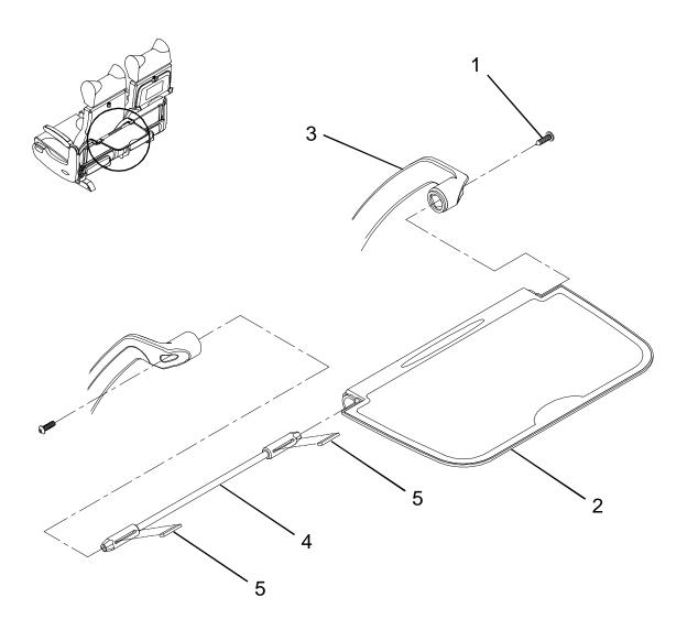
Figure 2-26 Tray Table Aircraft Style Top and/or Stopper Replacement
