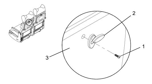
Figure 2-27 Tray Table Pivoting Hook Replacement
