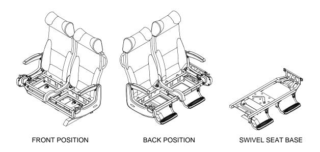
Figure 1-2 Two-Passenger Swivel Seat
