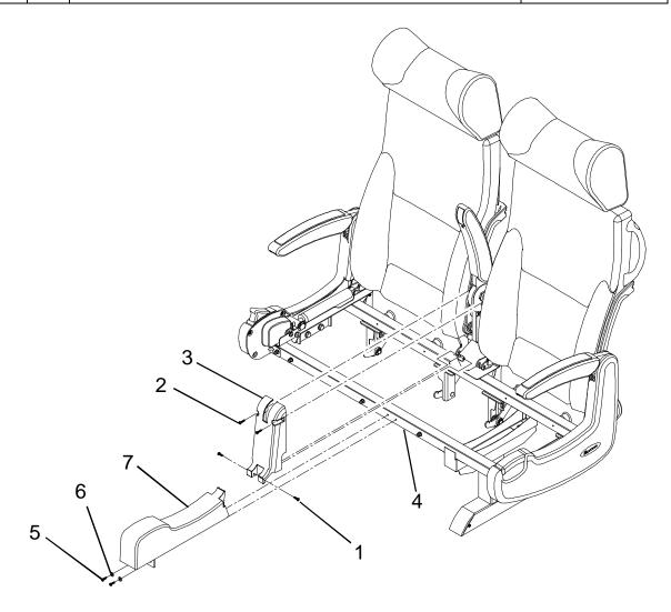
Figure 2-11 Center Front and Upper Shroud Replacement
