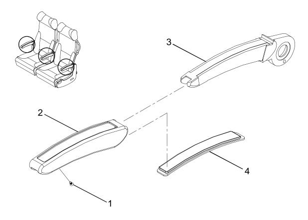
Figure 2-19 Armrest Cover and Foam Insert Replacement
