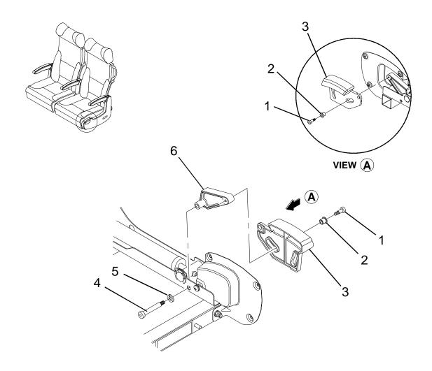
Figure 2-15 Reclining Handle and Lever Replacement
