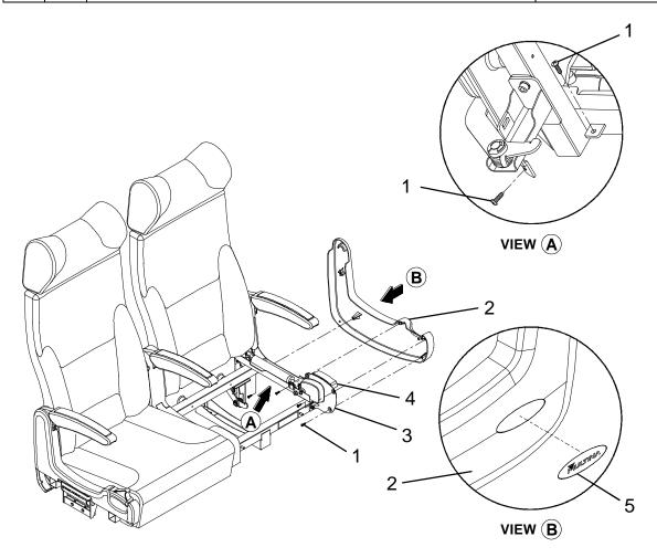
Figure 2-9 Aisle Side Shroud Replacement
