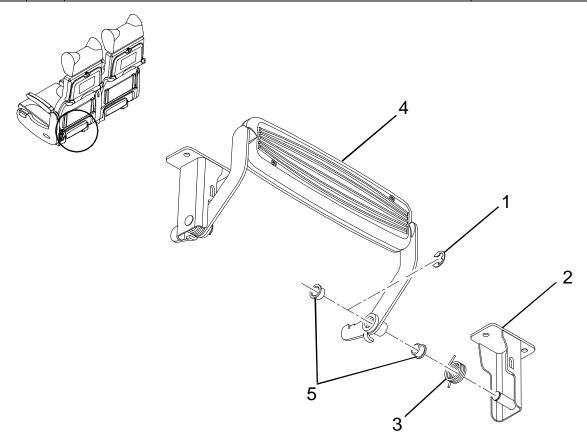
Figure 2-23 Footrest Torsion Springs and/or Flanged Bearings Replacement
