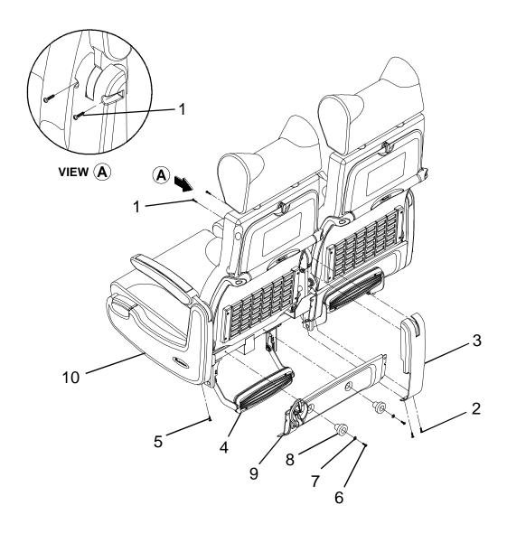
Figure 2-13 Footrest Bumper and Footrest Shroud Replacement
