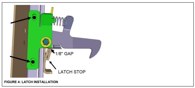
6. Secure the latch stop using two thread cutting screws #502848 (torque 10 lb-ft) (Figure 5). Apply torque seal mark.
