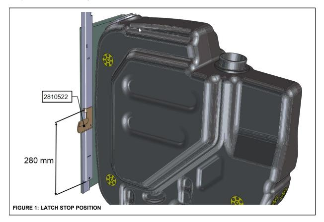
2. Secure the latch stop using two thread cutting screws #502848 (torque 10 lb-ft) (Figure 2). Apply torque seal mark.
