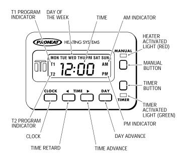
The Teleflex 7 Day Digital Timer can be preset for a single start time, one day at a time or two programmed start times per day constantly activated for multiple days of the week. The clock can be preset for 12 or 24 hour time display. The heater run time duration can be preset for 1 or 3 hours. The manual button can be used to override the program and run the heater indefinitely until it is switched off.
