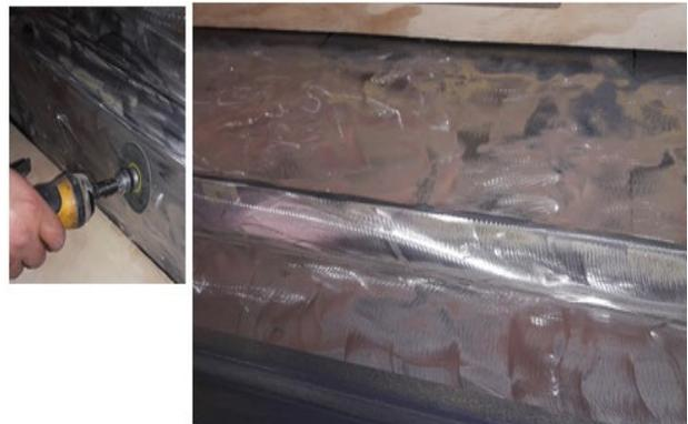
16. Sweep the wood floor so that remove dust and/or wood remains. Then use a wet cloth with thinner or alcohol to clean the plate.
