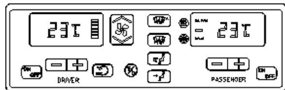
CENTRAL HVAC SYSTEM CONTROL MODULE
