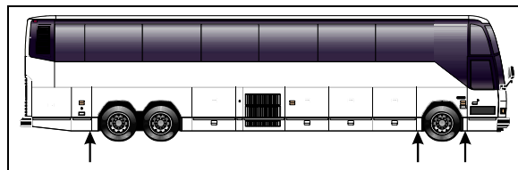
FIGURE 69: JACKING POINTS ON STRUCTURE 18302
