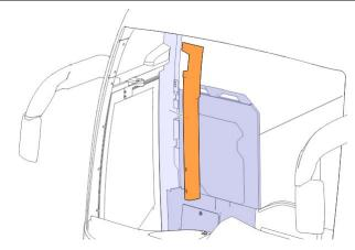
21. Pass the harness trough the air duct and route the harness to the electrical center on the pillar.
