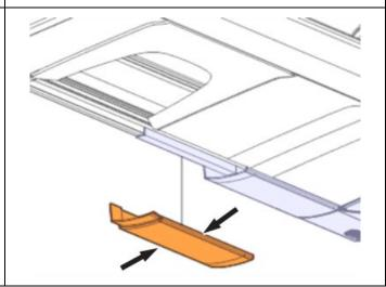
7. Mark the position of the sensors in the interior of the air condition duct.
