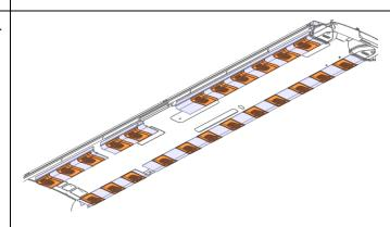
6. Remove the remaining panels, push the front and back part of the panel to loose them.
