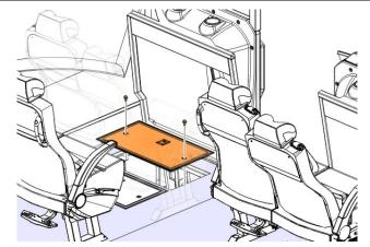
37. Install the panels on the luggage rack.Press the panel.
