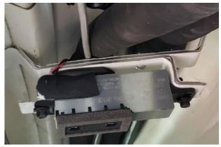
15. Use a 948995 connector, put the black cable on rounded side.
