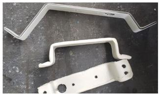
9. Join the brackets using the rivets included in the kit 24162097.
