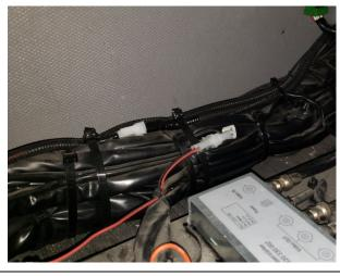
31. Cross the remaining harness under the stairs to the front electrical compartment on the right side.
