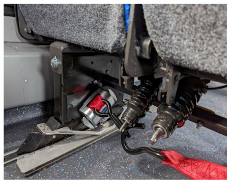
Figure 3: PIN MISSING
