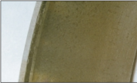
Peeling, the tearing away of metal from the race, the result of the breakdown of lubrication.
