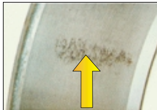
Etching of metal generally indicates water contamination, allowing oxidation to attack the surface.
