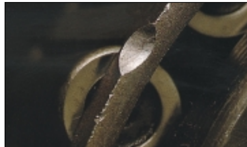
Cage damage, the result of abuse prior to or during installation.
