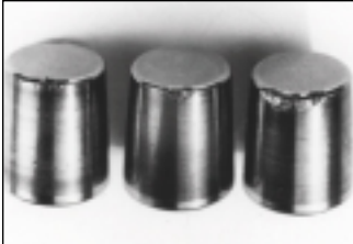
Roller end fracture due to heavy stress peaks caused by slackness of too loose bearing adjustment.
