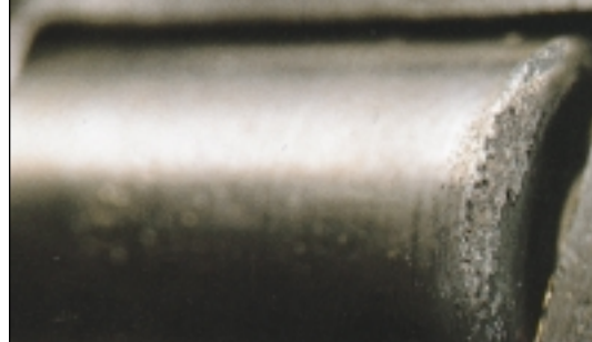
Large end of the roller shows spalling, the result of insufficient lubrication and/or excessive preload.
