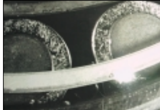
Roller end wear caused by over tightening, lubrication degradation, or lack of lubricant.
