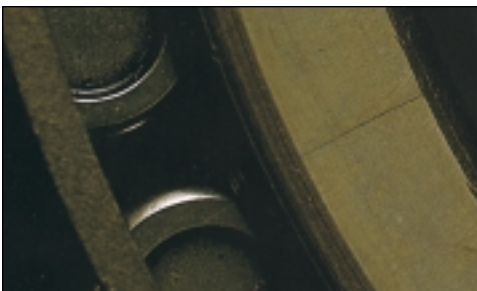
Cracked cone, the result of misapplication or cocking the cone at installation.
