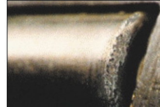
Roller end cracks indicate excessive loading or excessive misalignment.
