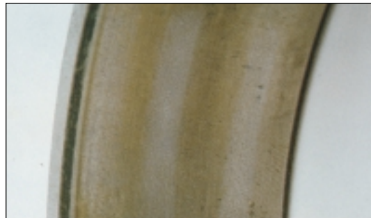
Pitting of the race, as a result of debris in the lube causing surface deformation.
