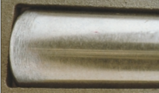
Large end of roller shows scoring, the result of excessive preload.
