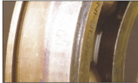
Discoloration indicates high levels of heat, the result of improper lubrication or improper bearing adjustment.
