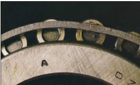
Deformation of the cage, the result of improper installation or mishandling prior to installation.
