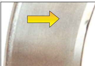
Dings and dents in the bearing surfaces indicates a drift was used during installation.
