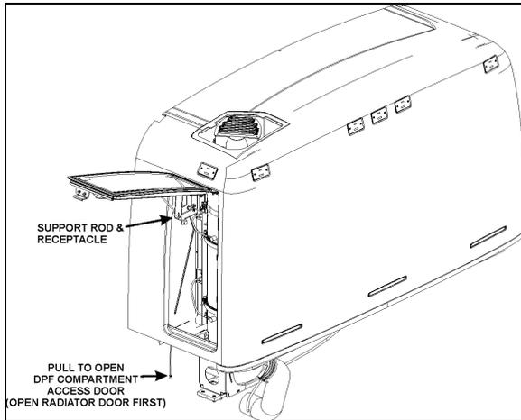
ACCESS TO THE CATALYTIC CONVERTER
