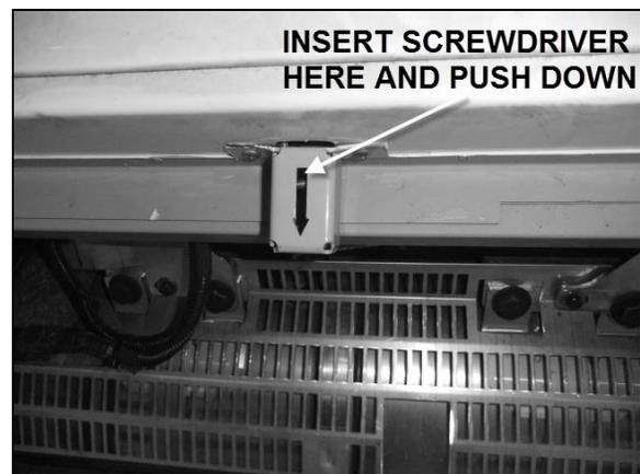
To close the door, lower the door and push against the release lever spring to latch the door shut.
