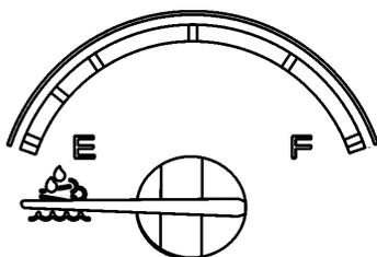
Indicates the amount of DEF (Diesel Exhaust Fluid) remaining in the DEF tank. The DEF tank is considered as being full when it contains 16 gallons (60 liters) of DEF. DEF consumption will be approximately 2% of the diesel fuel consumed.
