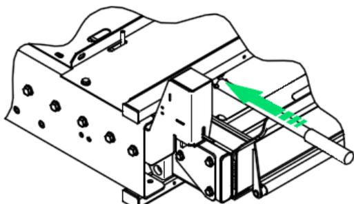
3. Turn the manual platform release shafts counterclockwise using manual backup pump handle extension to disengage the platform and then lift the stowlock mechanical catch.
