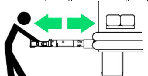
5. Turn the manual platform release shafts using pump handle extension back to previous position to lock the platform.
