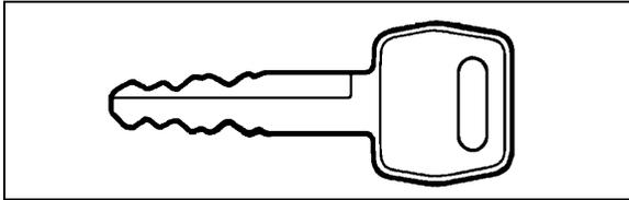
Use one of the two exterior compartment keys provided to lock or unlock any exterior compartment door, including the electrical or service compartment doors, but excluding the fuel tank filling access doors. It is also possible to lock or unlock the baggage compartments and service compartments from the inside by means of a switch located on the dashboard.
