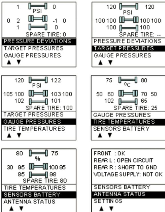
The display remains in this mode with the menus appearing at the bottom until the pre-trip check sequence starts again.
