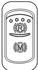
Use this switch to select between the transmission retarder and the engine brake when using the vehicle speed retarding device switches on the steering wheel. Both systems cannot be in function at the same time. This rocker switch will be found on the dashboard only if the vehicle is equipped with both systems. Refer to "Transmission Retarder" heading in this chapter. Refer also to "Transmission Retarder" & "Engine Brake" in "OTHER FEATURES" chapter.
