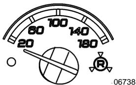
Indicates the rear brake air system pressure in psi. The normal operating pressure is from 122 to 140 psi.
