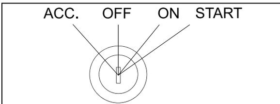
The ignition switch doubles as the battery master switch. Any position other than OFF activates the battery electrical circuit. The battery electrical circuit is also activated when the hazard switch is depressed.
