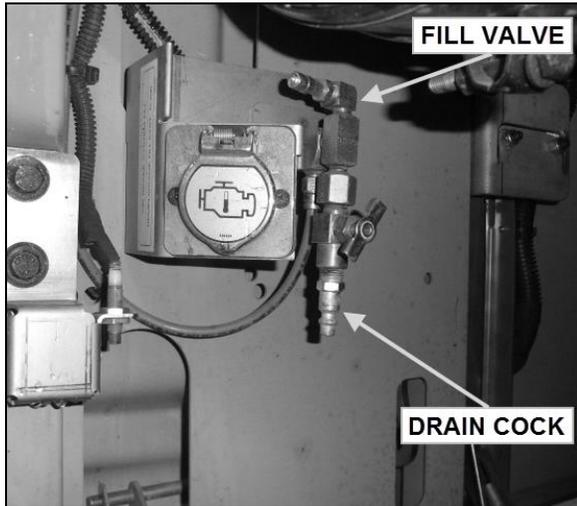
FILL VALVE IN ENGINE COMPARTMENT 12162
