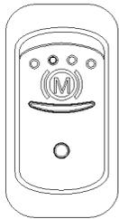
The vehicle's engine brake is by default set to automatic (AUTO mode (A)). On vehicles equipped with this switch, it is possible to disable the engine brake (OFF mode).
