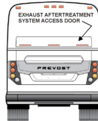
The engine door must be open before opening the exhaust aftertreatment system access door. To open the access door, lower the latch release lever, using a flat tip screwdriver.
