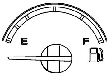
Indicates the amount of fuel remaining in the fuel tank. At the beginning of the red area, there is approximately 48 gallons (182 liters) left in the tank.
