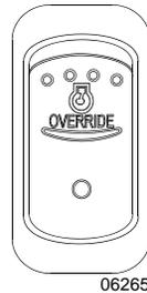
Press the Engine Stop Override switch on the dashboard or the Delay Engine Stop switch on the AFSS protection panel to delay the engine shutdown and extinguisher discharge by an additional 15 seconds.
