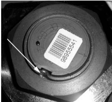
FIGURE 13: FIXING NUT PUNCH MARK
