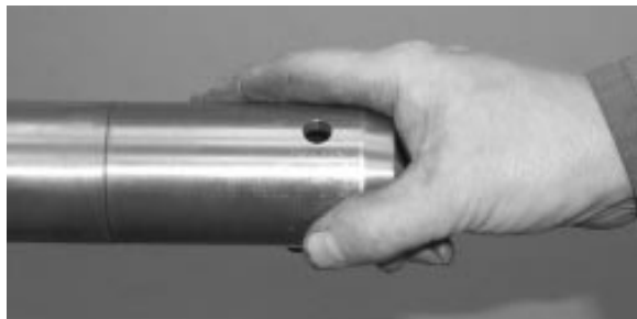
FIGURE 9: OUTIL D'INSERTION N/P PREVOST 491115
