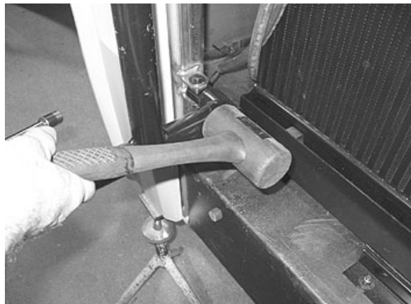
FIGURE 63: PANTOGRAPH ARM ADJUSTMENT
