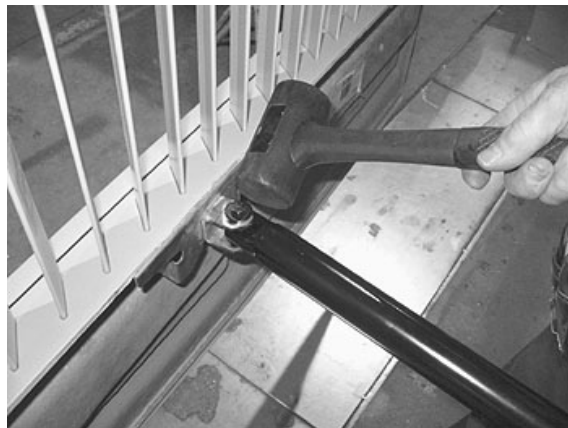
FIGURE 64: DOOR LATERAL ADJUSTMENT
