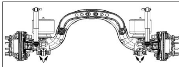
FIGURE 85: JACKING POINTS ON TAG AXLE
