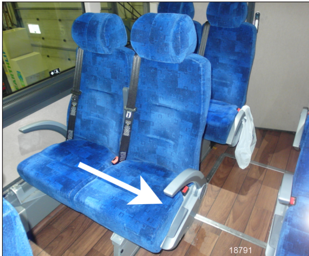
PULL TO UNLOCK THE ROTATION
