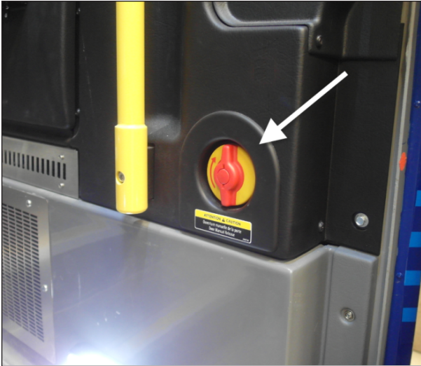
INTERIOR UNLATCH AIR VALVE
