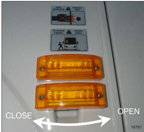
FIGURE 23: ENTRANCE DOOR EXTERIOR SWITCH – H3
