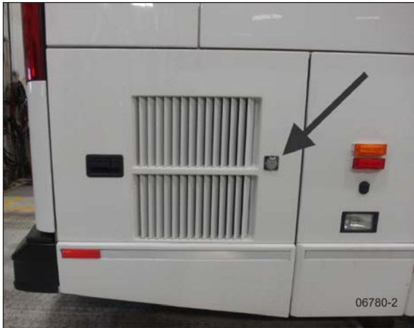
FIGURE 28: BATTERY CHARGER 120-VOLT CONNECTOR – H3
