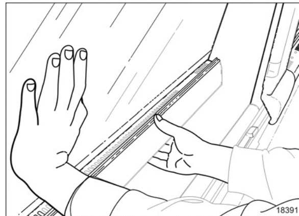
EMERGENCY WINDOW OPENING
