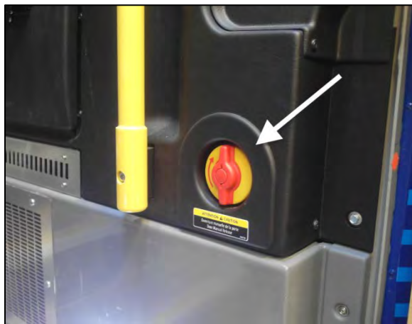
INTERIOR EMERGENCY RELEASE AIR VALVE 12164
