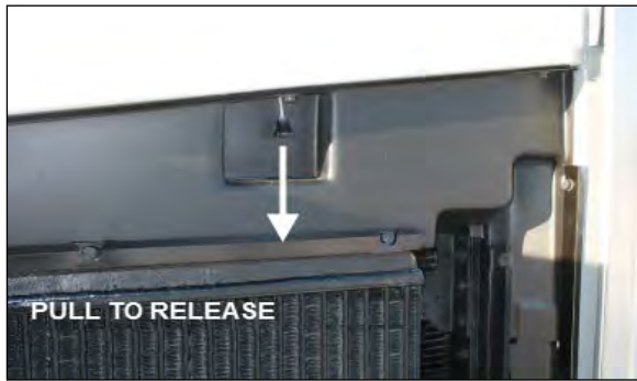
UNLOCKING SCR CONVERTER ACCESS DOOR
