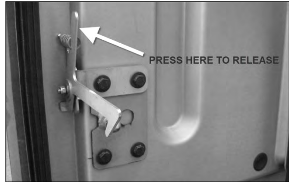
EVAPORATOR COMPARTMENT DOOR SECONDARY LOCK LEVER
