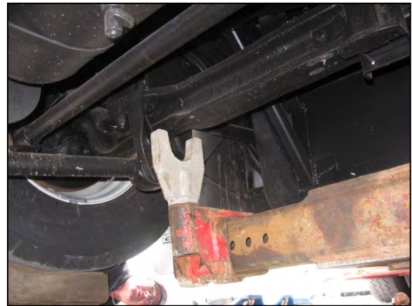
LIFTING FROM UNDER THE FRONT AXLE
