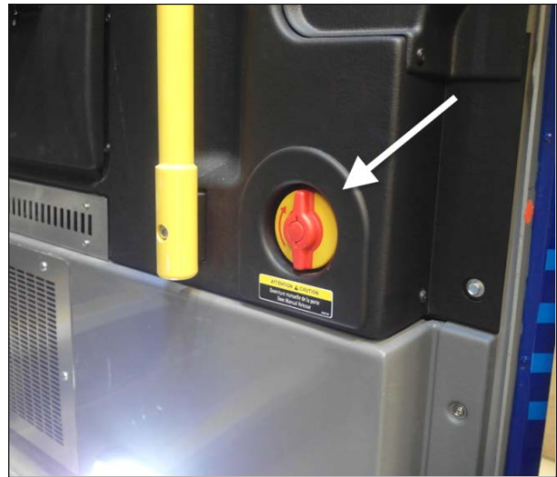
INTERIOR UNLATCH AIR VALVE
