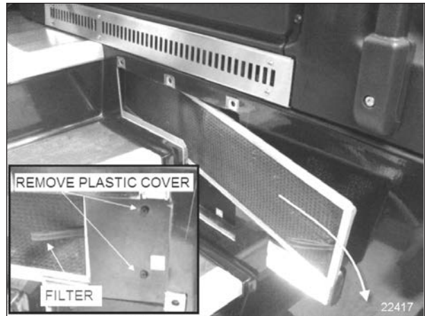
REMOVING DRIVER'S SECTION AIR FILTER
