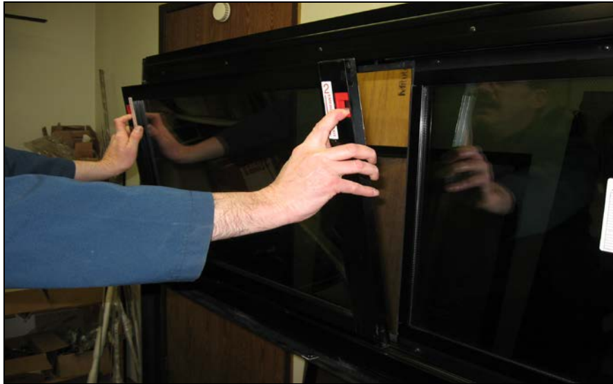
FIGURE 95: REMOVING THE SASH
