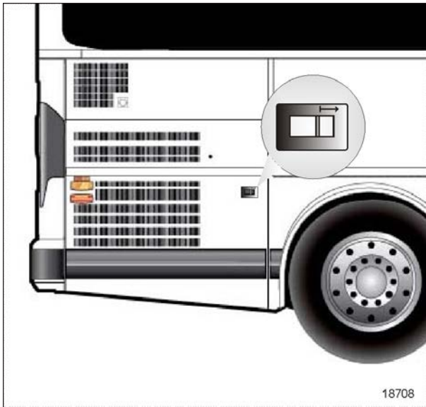
ENGINE COMPARTMENT CURBSIDE DOOR
