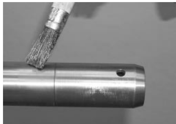
FIGURE 19: APPLY GLEITMO 805 GREASE
