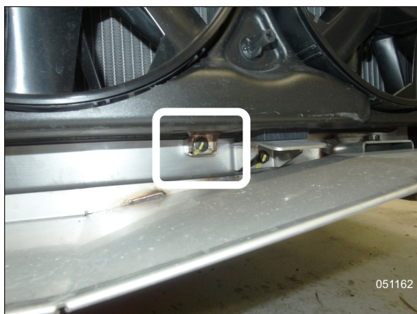
FAN SHROUD TOP & BOTTOM HOLD-DOWN SCREWS
