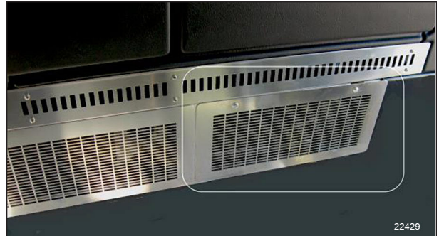
DRIVER'S AREA AIR FILTER GRILL REMOVAL
