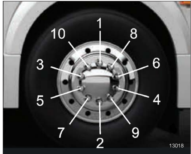
FIGURE 14: TIGHTENING SEQUENCE
