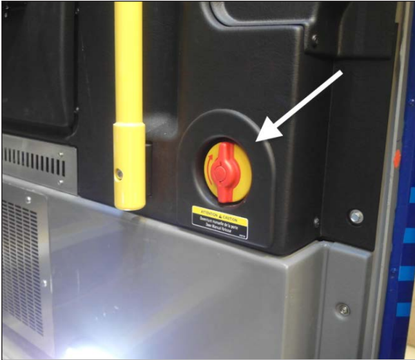
FIGURE 6: INTERIOR UNLATCH AIR VALVE
