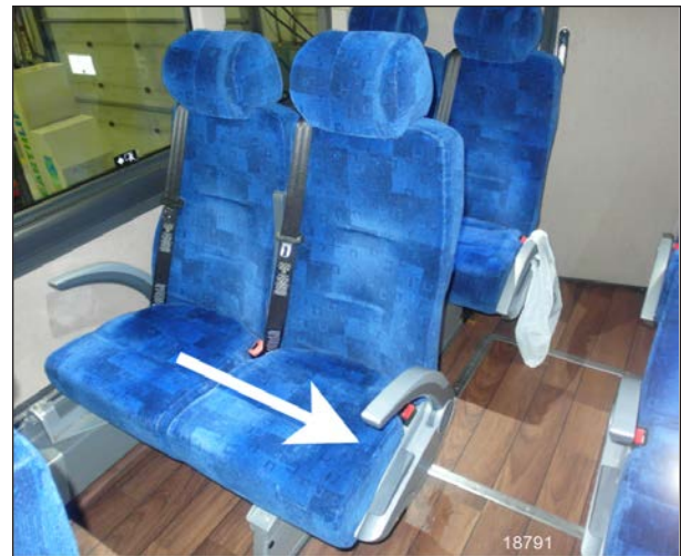
FIGURE 12: PULL TO UNLOCK THE ROTATION
