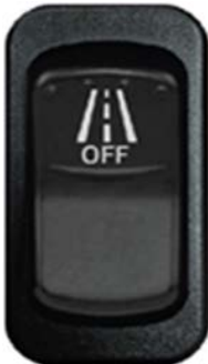
FIGURE 17: LDW ENABLE/DISABLE SWITCH
