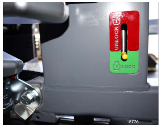
FIGURE 17: SECONDARY LOCK INDICATOR
