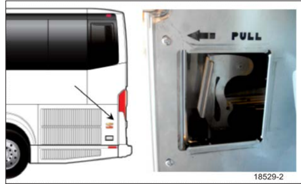
FIGURE 8: RADIATOR DOOR LATCH RELEASE LEVER LOCATION
