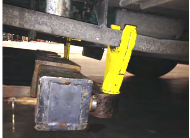
Figure 68: PROPER LOCATION WHEN LIFTING THE SIDE-MEMBERS
