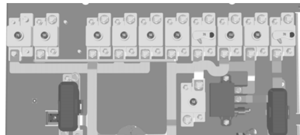
FIGURE 17: MAIN CIRCUIT BREAKERS IN MPC
