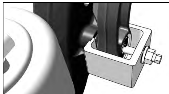
FIGURE 6: INSTALLING EXTRACTOR TOOL
