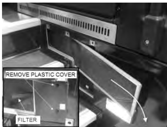
FIGURE 9: REMOVING DRIVER'S SECTION AIR FILTERS
