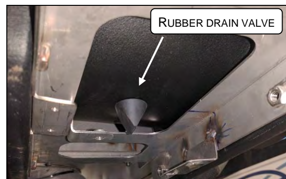
FIGURE 26 RUBBER DRAIN VALVE UNDER FILTER
