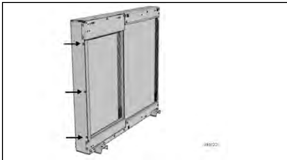
FIGURE 49: CAC LATERAL SUPPORT BOLTS
