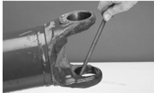
FIGURE 20: RAISED METAL OR FRETTING CAN BE REMOVED FROM YOKE CROSS HOLES WITH A FINE-TOOTHED FILE
