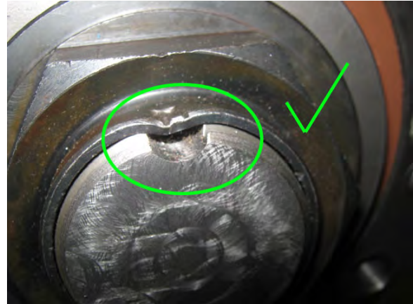
FIGURE 23: CORRECT - PREVENTS THE NUT FROM GETTING LOOSE
