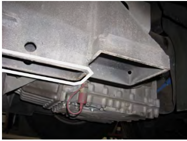
FIGURE 2: CHASSIS HOISTING POINTS - AFT OF TAG AXLE
