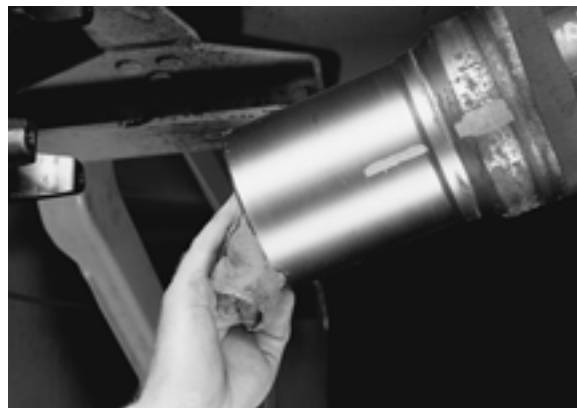
FIGURE 22: CLEAN GREASE FROM SPLINE SLEEVE
