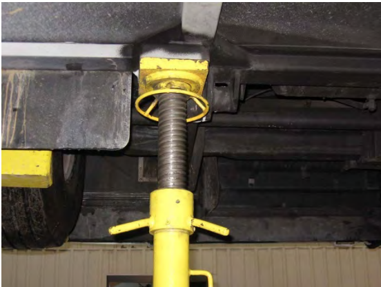
FIGURE 5: JACK STAND AT CHASSIS HOISTING RECEPTACLE - AFT OF FRONT AXLE, ROAD SIDE
