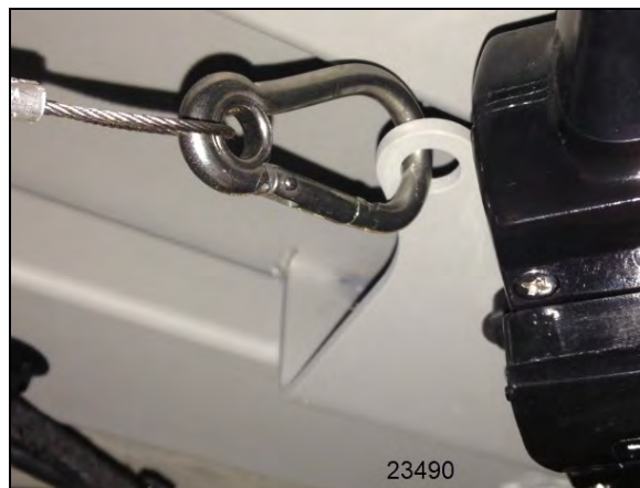
FIGURE 21: PROTECTIVE WIRE INSTALLATION
