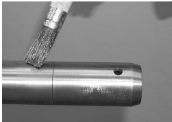
FIGURE 18: APPLY GLEITMO 805 GREASE
