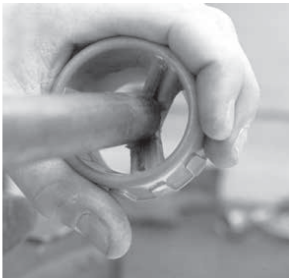
FIGURE 14: DEBURR THE TUBE END - OUTER
