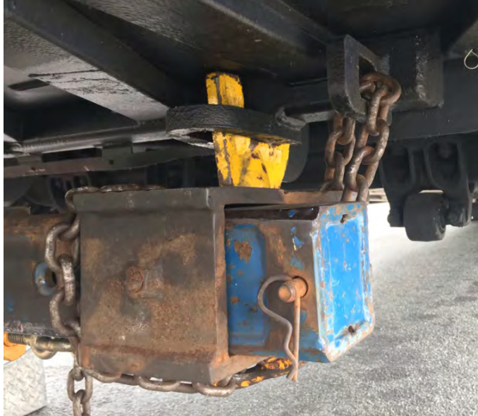
Figure 41: DOB BUS NUMBER SERIES 1300–1606 CHOKE CHAINS ROUTING
