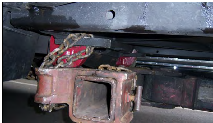
Figure 40: DOB BUS NUMBER SERIES 2400–2489 & 2490–2789 CHOKE CHAINS ROUTING
