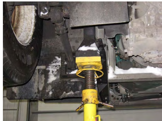
FIGURE 8: JACK STAND AT CHASSIS HOISTING RECEPTACLE - AFT OF TAG AXLE, CURB SIDE
