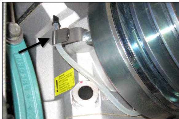
FIGURE 17: SHAFT SEAL OIL COLLECTING TUBE
