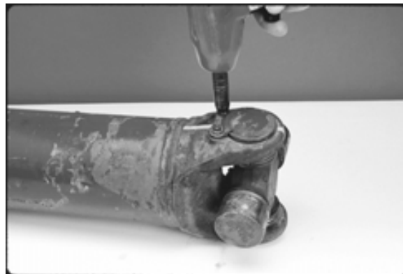
FIGURE 15: SPRING TAB BOLTS REMOVAL
