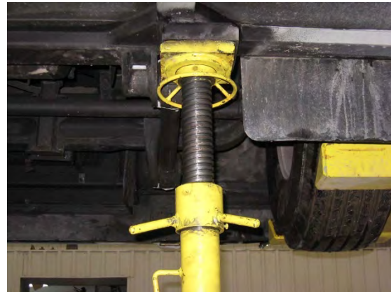
FIGURE 6: JACK STAND AT CHASSIS HOISTING RECEPTACLE - AFT OF FRONT AXLE, CURB SIDE
