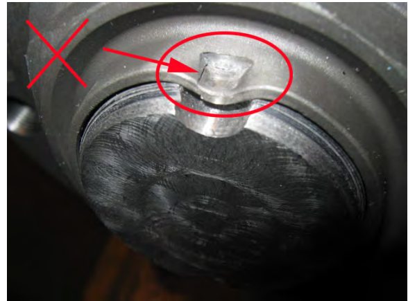
FIGURE 25: BROCKEN OR TORN LIP – REJECTED
