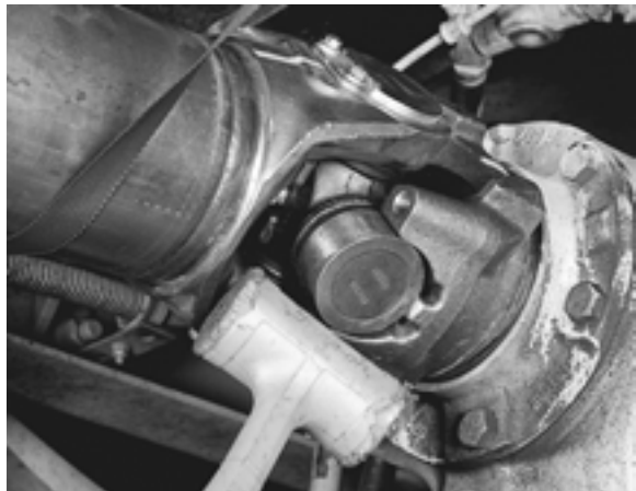
FIGURE 13: UNSEATING BEARING CUP ASSEMBLIES
