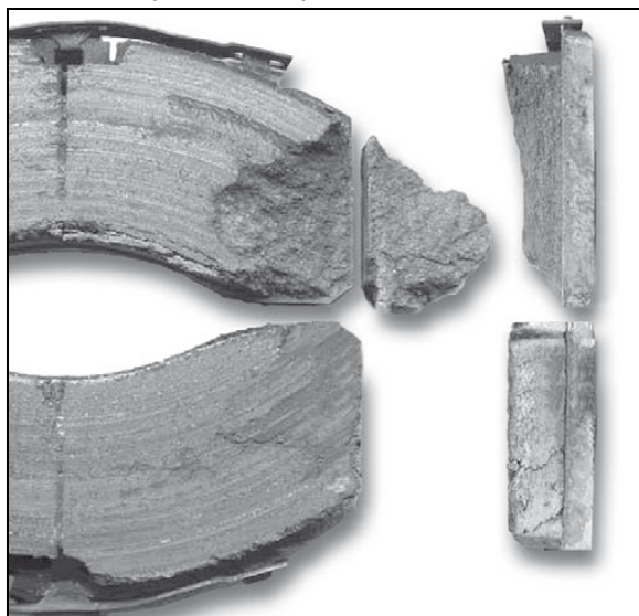
FIGURE 29: MAJOR BREAKOUTS ON THE SURFACE OF THE BRAKE PAD ARE NOT PERMITTED
