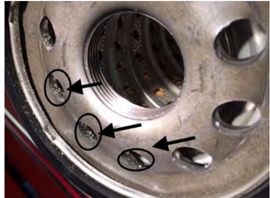
ALUMINUM PARTICLES FOUND ON A PRE-GHG17 FILTER CAUSED BY GRINDING OF THE TOP OF THE FILTER INTO THE FILTER RESTRICTOR
