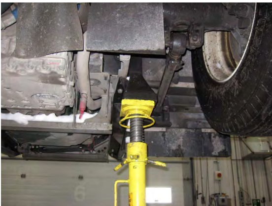
FIGURE 7: JACK STAND AT CHASSIS HOISTING RECEPTACLE - AFT OF TAG AXLE, ROAD SIDE
