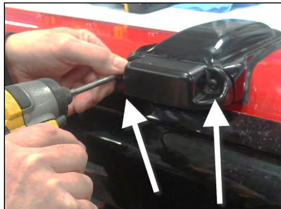
FIGURE 81: PERIMETER LIGHT DISASSEMBLY 2. Disconnect light.
