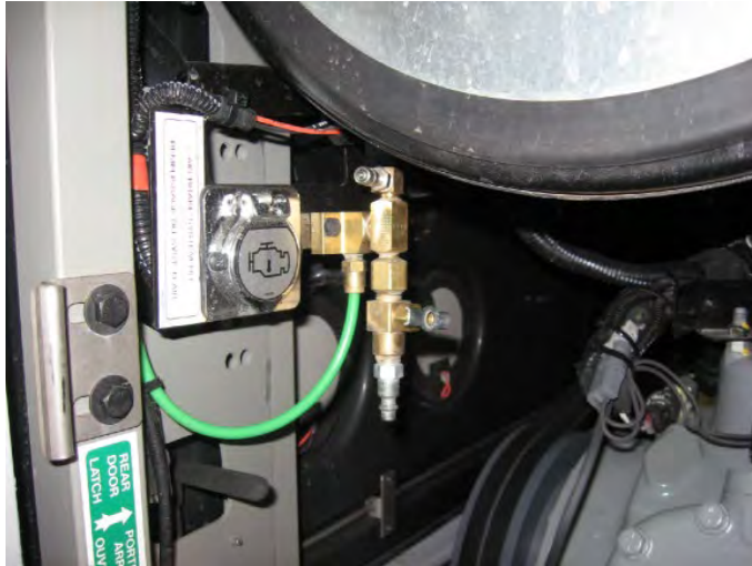
Figure 23: ENGINE COMPARTMENT EMERGENCY AIR-FILL VALVE
