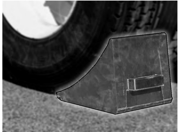
Figure 19: CHOCK THE FRONT AND REAR WHEELS
