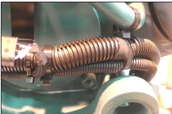
Figure 13: starter cables in a corrugated protective sheath.
