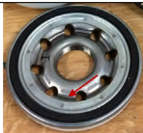
GHG17 END CAP DESIGN WITH DEEP GROOVE
