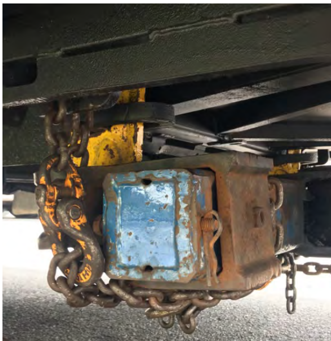
Figure 43: : DOB BUS NUMBER SERIES 1300–1606 CHOKE CHAINS ROUTING
