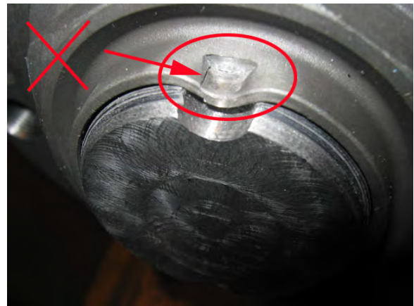
FIGURE 25: BROCKEN OR TORN LIP – REJECTED
