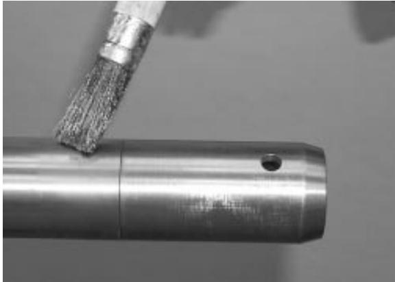
FIGURE 18: APPLY GLEITMO 805 GREASE
