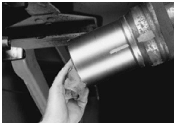
FIGURE 22: CLEAN GREASE FROM SPLINE SLEEVE
