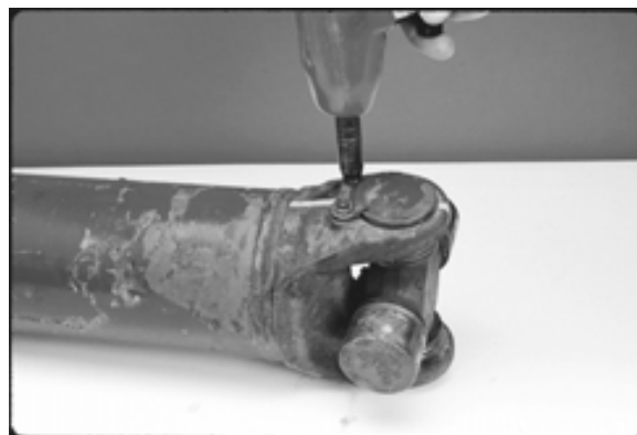
FIGURE 15: SPRING TAB BOLTS REMOVAL
