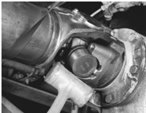
FIGURE 13: UNSEATING BEARING CUP ASSEMBLIES
