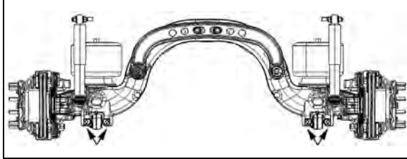
FIGURE 5: JACKING POINTS ON TAG AXLE 11023
