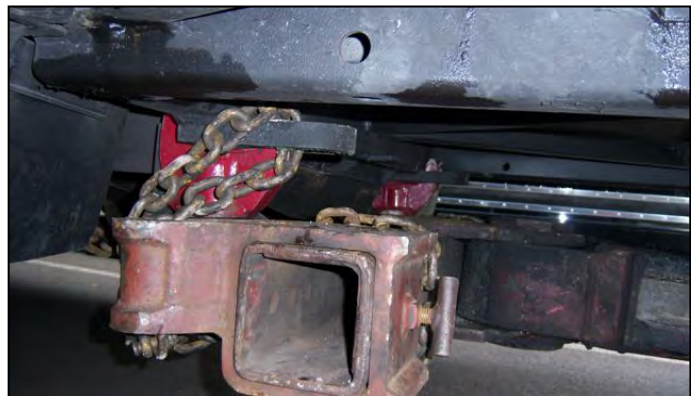
Figure 40: DOB BUS NUMBER SERIES 2400–2489 & 2490–2789 CHOKE CHAINS ROUTING
