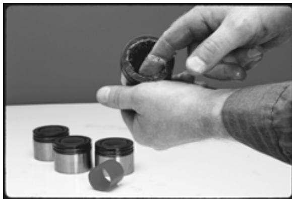
FIGURE 27: GREASING BEARING CUP
