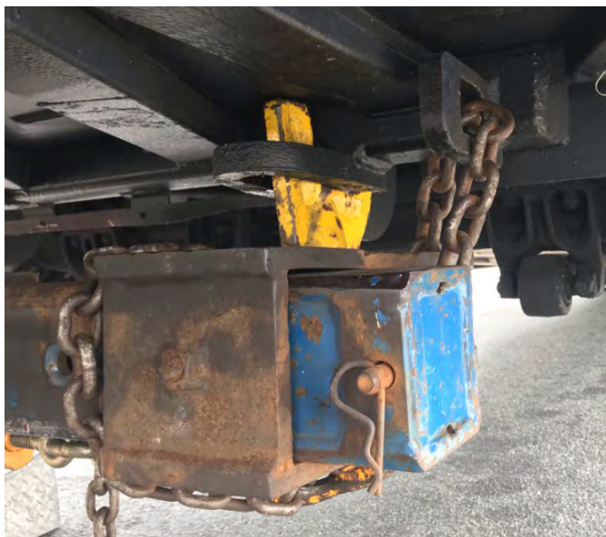
Figure 41: DOB BUS NUMBER SERIES 1300–1606 CHOKE CHAINS ROUTING
