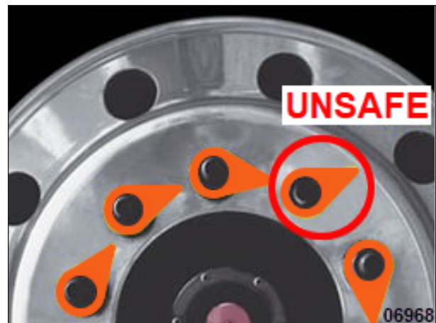
FIGURE 15: LOOSE WHEEL NUT INDICATORS - UNSAFE DRIVING CONDITION
