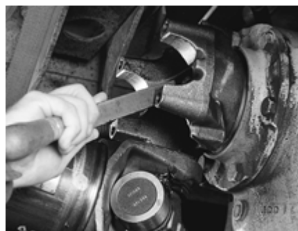
FIGURE 16: RAISED METAL OR FRETTING ON OPEN YOKE CROSS HOLES
