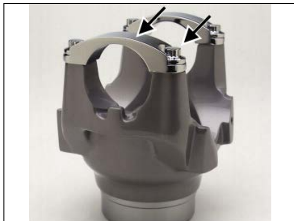
FIGURE 2: COLD FORMED BEARING RETAINER AND BOLTS AS USED ON PREVOST VEHICLES
