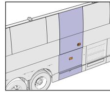
To open the optional wheelchair lift door, the coach must be parked on a flat and level surface with the parking brake applied. The wheelchair access door swings to the side and is maintained open by a locking mechanism. Open the baggage compartment containing the lift mechanism. The baggage compartment door is located directly below the wheelchair access door and it opens to the side.
