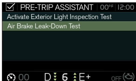
The Air Brake Leak-Down Test check allows the driver to accurately measure the amount of air pressure drop in the front and rear brake air systems. After selecting this test from the DID, you are prompted to apply the service brake for 60 seconds. After applying and holding the service brake for 60 seconds, the DID will display the amount of pressure drop in the brake system.
