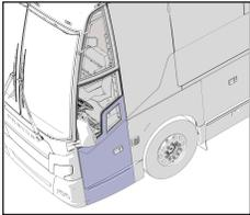
Unlock this compartment door using the exterior compartment key. The light in the front service compartment turns on automatically when the door is open.
