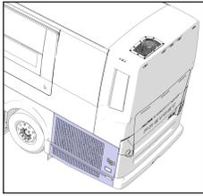
Open the engine compartment rear door to access the engine radiator door release handle.
