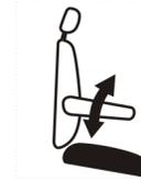
To lower or raise the seat's rear section, pull the handle #4 up and push or pull the seat cushion.
