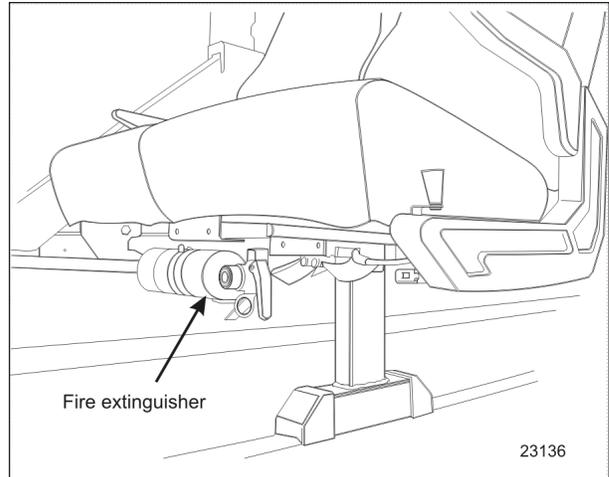
FIGURE 7: FIRE EXTINGUISHER UNDER FIRST ROW SEAT
