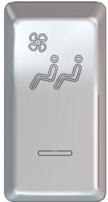
Press this switch to activate the passenger overhead air registers fan.
