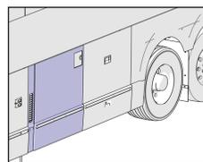
To access the evaporator compartment, pull the release latch located on the left side wall of the rearmost baggage compartment.
