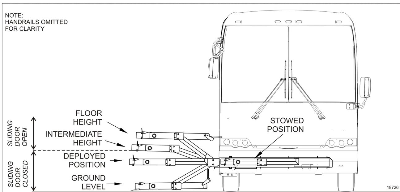
**FIGURE 9: PLATFORM POSITION WITH INTERMEDIATE HEIGHT (OPTIONAL FEATURE)**
