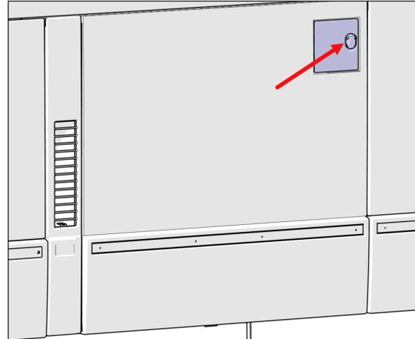
**FIGURE 29: FUEL FILLER NECK ACCESS HATCH LOCK**
