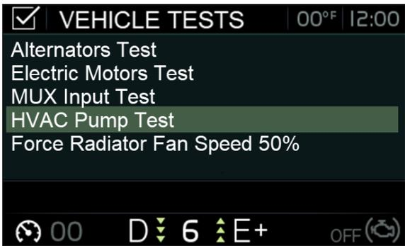
In test mode, with the parking brake applied and the passenger set point set to a value higher than 64°F (18°C), the circulator pump is not set to OFF as it would normally do when the outside temperature gets above 50°F (10°C). This feature allows verification of the pump when inside a garage. This is also useful when working on the heating system to remove air pockets trapped in the system.
