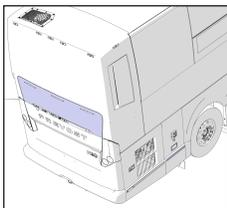
The engine compartment door must be opened before opening the DPF access hatch. To open, press the latch release lever. Using both hands, push the access hatch up until it locks in place.
