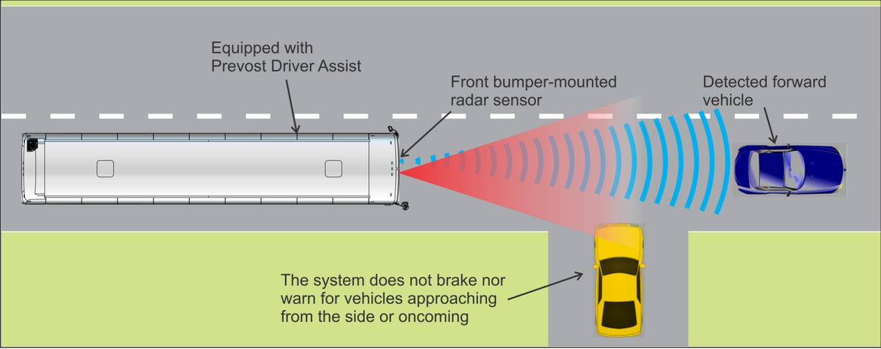
Equipped with Prevost Driver Assist
