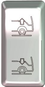
Momentarily press the rocker switch downwards to lower the front end of the coach 4 inches (100 mm). Momentarily press the rocker switch upwards to raise the coach to the normal driving height. Refer to ["High-BUOY" on page 14](#) and ["KNEELING SYSTEM" on page 1](#) in Section 5 for more information.
