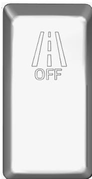
FIGURE 42: LDW ENABLE / DISABLE SWITCH
