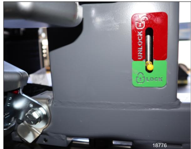
**FIGURE 19: SECONDARY LOCK INDICATOR**
