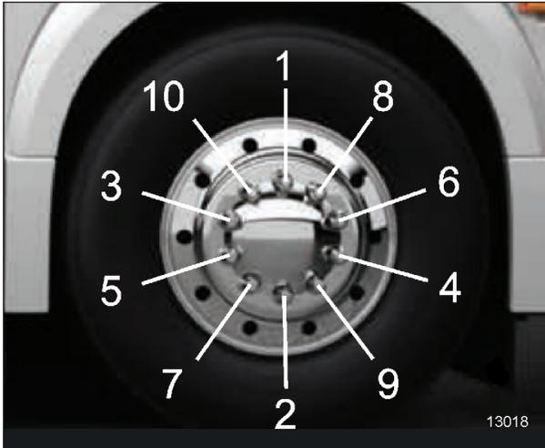
FIGURE 13: TIGHTENING SEQUENCE
