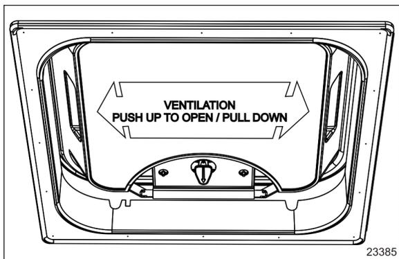
FIGURE 17: VENTILATION HATCH
