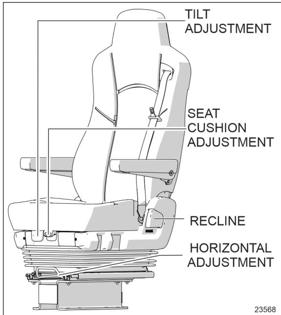
FIGURE 4: PNEUMATIC DRIVER'S SEAT
