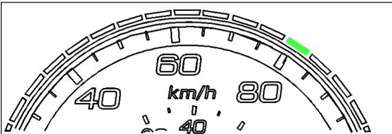
FIGURE 48: THE CRUISE SET SPEED IS 80 KM/H
