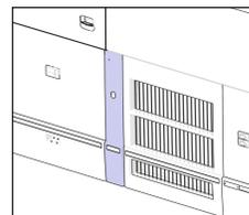
Open this door using the exterior compartment key. To open, turn the key ¼ turn clockwise and pull the door open.
