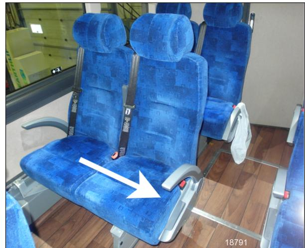
**FIGURE 10: PULL TO UNLOCK THE ROTATION**
