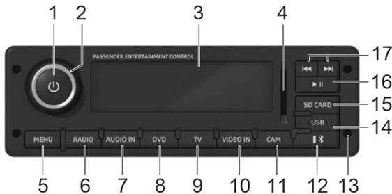
The VSS-06 Video and Sound Selector enables the driver to select audio, audio/video and video sources with settings of volume level, bass, treble, loudness for the passenger's area only. The DVD player, media player, microphones and auxiliary audio or video sources are controlled with this unit.
