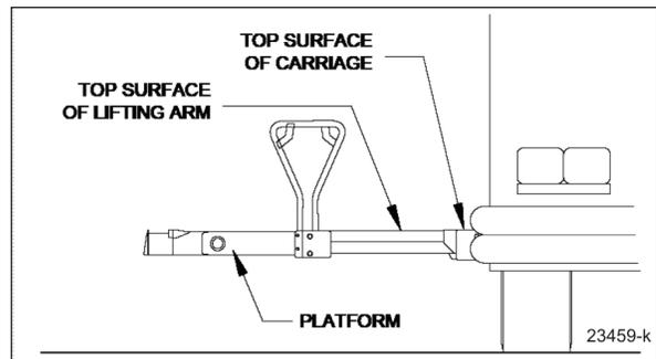
FIGURE 14: LIFTING ARM AND CARRIAGE AT SAME HEIGHT
