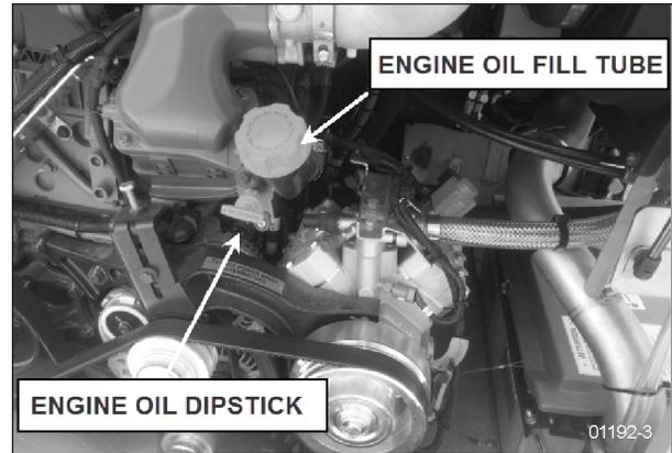
FIGURE 4: ENGINE OIL DIPSTICK - VOLVO D13 ENGINE
