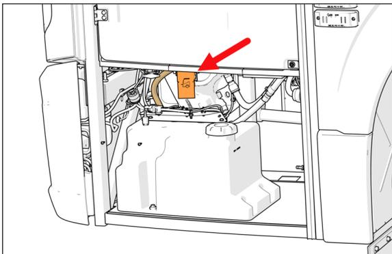
**FIGURE 20: WIPERS MECHANISM ACCESS HATCH
