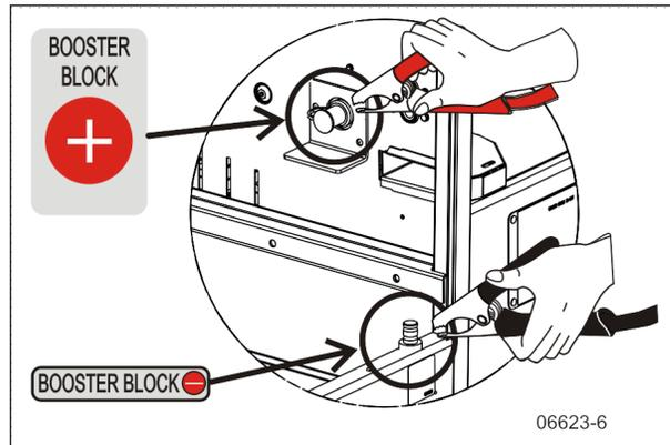
FIGURE 4: BOOSTER BLOCK TERMINALS LOCATION (H3 SERIES)
