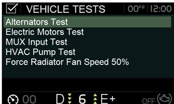
This feature will activate one alternator at a time during 5 seconds, cycling between alternator 1, 2 & 3.
