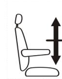
Pull both handles (3 and 4) up to adjust the height of the seat.
