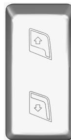
Use this rocker switch to open or close the driver's power window.
