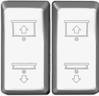
Press and hold the appropriate button to lower the left or right windshield sunshades. Press twice rapidly to raise or lower up to the end position.
