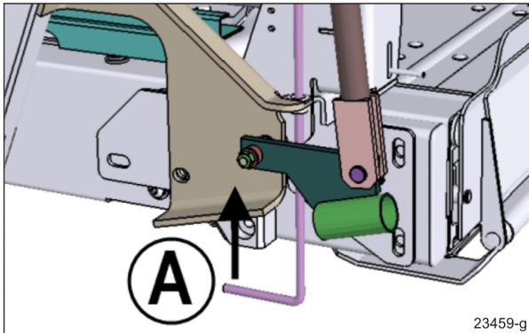
4. Pull rollstop control knob out and rotate fully counterclockwise. Rollstop must lie flat on ground.
