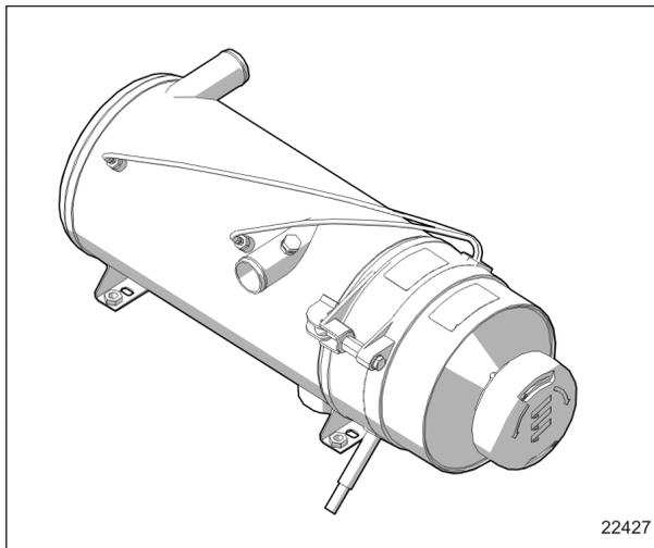
**FIGURE 5: COOLANT PREHEATER**
