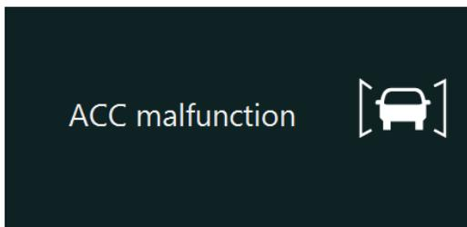
ACB SENSOR (RADAR) BLOCKED
