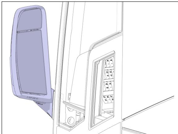
To provide good visibility in cold weather, the mirrors can be equipped with heating elements. The elements are activated by a rocker switch located on the dashboard. Refer to "Controls & Instruments" chapter. Thermostats are used to prevent continuous operation of the heating elements.
