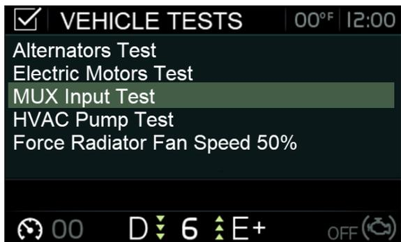
In VEHICLE TESTS, select MUX INPUT TEST. Press ENTER / SELECT button to start the test.
