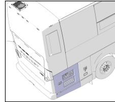
Lock this door using the exterior compartment key. To open, pull up the door handle to release the latch and then pull the door open.
