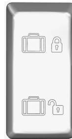
This system enables locking all baggage compartment doors by pressing the switch forward. To unlock, press the switch rearward.
