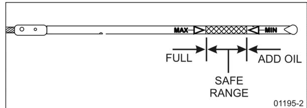
FIGURE 5: VOLVO D13 ENGINE OIL LEVEL DIPSTICK
