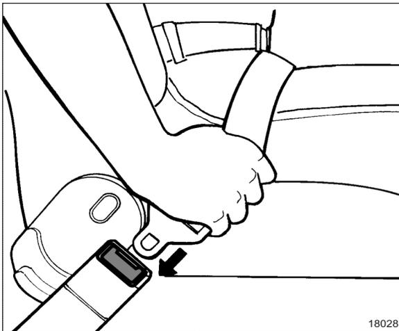
**FIGURE 6: TO FASTEN SEAT BELT**
