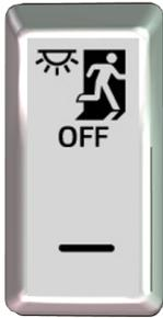
Use this switch to reset the Emergency Lighting System once it was triggered either by a real accident, by a big hit of the vehicle which led to a false trigger of the system or either due to a test of the system.
