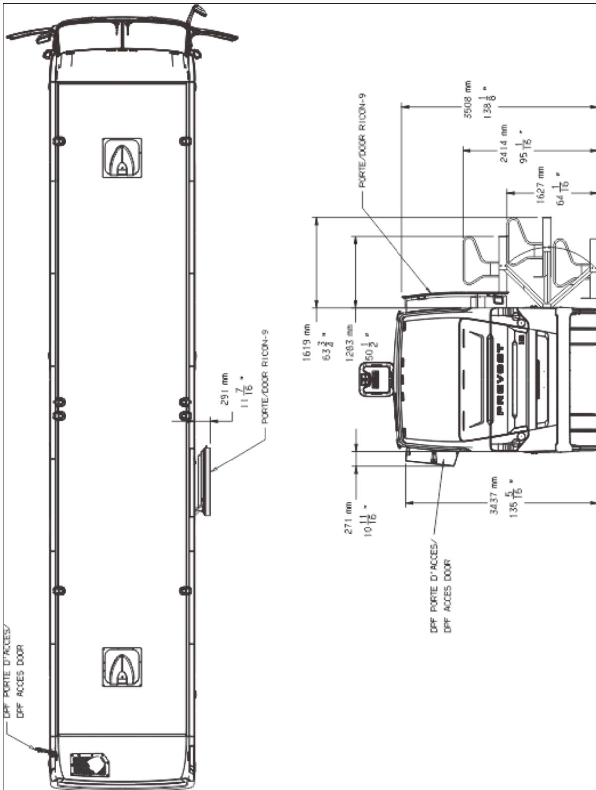
FIGURE 3: H3 SERIES WITH WHEELCHAIR LIFT - OVERALL DIMENSIONS
