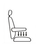
For maximum mechanical suspension performance, rotate the handwheel #6 until your body weight (in pounds) is shown on the indicator.
