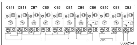
**FIGURE 11: MAIN CIRCUIT BREAKERS 12 & 24 VOLTS (TYPICAL)**
