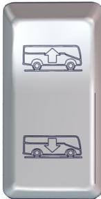
Press and hold this rocker switch to raise or lower the coach about 4 inches (100 mm). Release the rocker switch to return the coach to the normal driving height.
