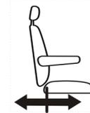
To adjust distance between driver and dashboard, pull the handle #5 up and slide the seat forward or backward.
