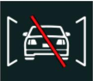
FORWARD VEHICLE DETECTED - MISSING/ERROR STATE pictogram
