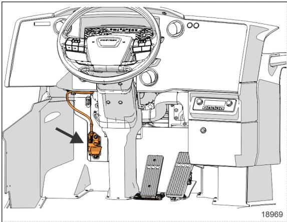
FIGURE 34: STEERING WHEEL TILT AND TELESCOPIC ADJUSTMENT
