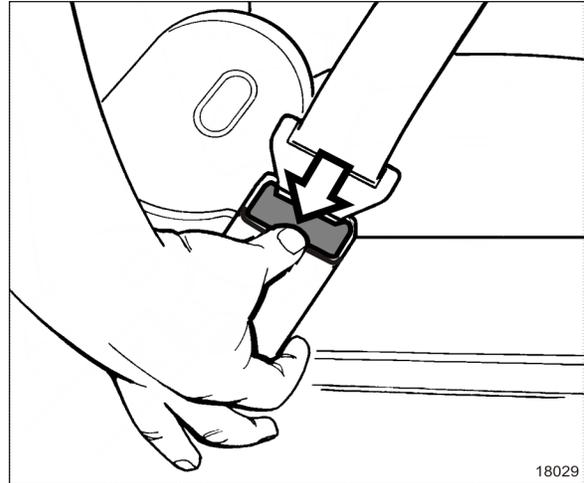
**FIGURE 7: TO UNFASTEN SEAT BELT**
