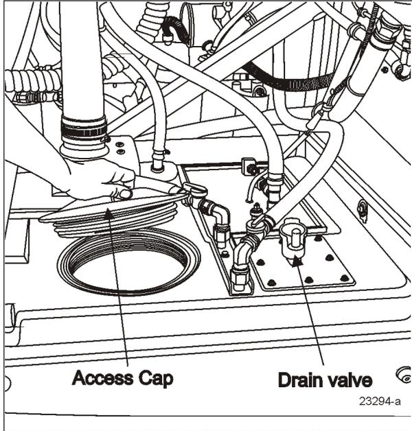
FIGURE 1: SINGLE LAVATORY WASTE WATER TANK OPTION
