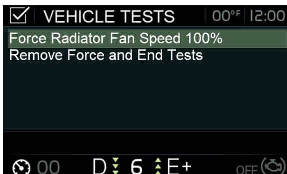
Prerequisite condition: The engine is running (fast idle if at stand still).
