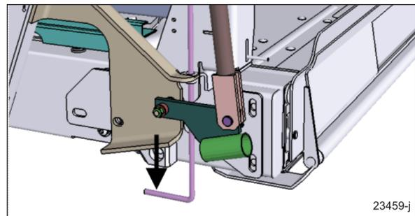
2. Raise the platform to stow height; position the top surface of the platform lifting frame arm at the same height as the top surface of the carriage. If the exact height cannot be obtained, a slightly low platform is preferred to slightly high. This alignment eliminates interference between the platform and enclosure when pushing the platform into the enclosure.
