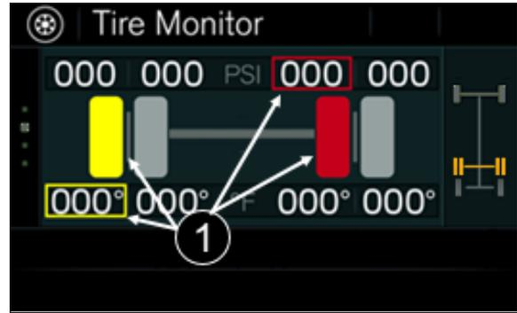
FIGURE 36: READING PRESSURE AND TEMPERATURE ON ON DRIVE AXLE TIRES WITH IRREGULARITIES DETECTED (DISPLAY EXAMPLE)
