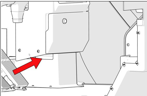
**FIGURE 21: ACCESS TO THE RECIRCULATING AIR FILTERS**
