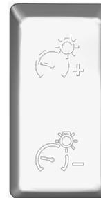
Adjust the brightness of the dashboard instruments and switches.
