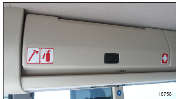
FIGURE 7: A DECAL INDICATES THAT A FIRE HATCHET, A FIRE EXTINGUISHER AND A FIRST-AID KIT ARE LOCATED IN THIS OVERHEAD COMPARTMENT
