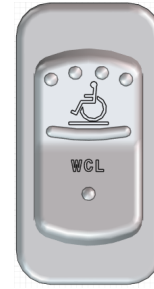
FIGURE 9: WHEELCHAIR LIFT POWER SWITCH
