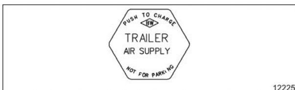
The trailer air braking system is supplied by pushing this control valve.
