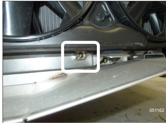
FIGURE 14: VIS DE MONTAGE DU CARÉNAGE DES VENTILATEURS
