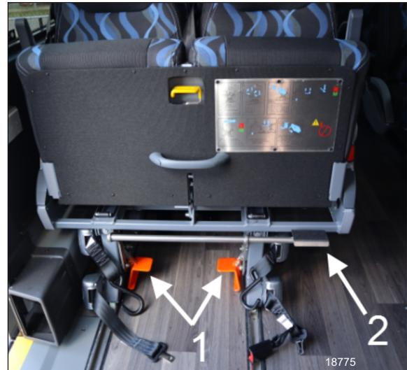
FIGURE 16: DÉPLACEMENT DE SIÈGE COULISSANT
