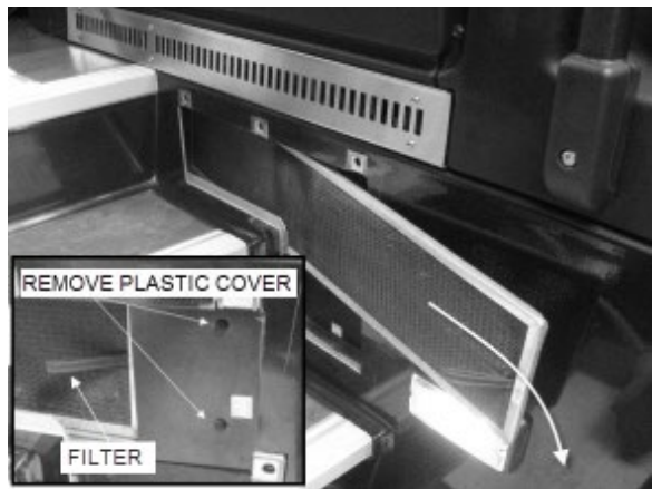
FIGURE 18: REMOVING DRIVER'S SECTION AIR FILTERS
