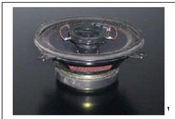
FIGURE 10: 10CM COAXIAL SPEAKER
