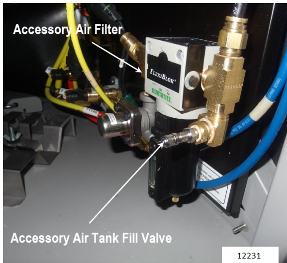
FIGURE 4: FRONT SERVICE COMPARTMENT
