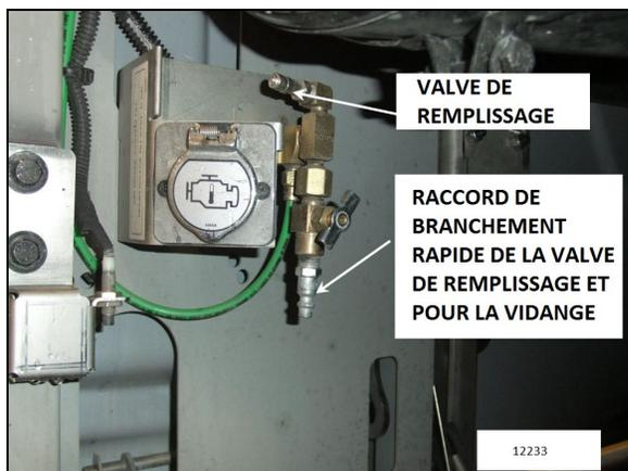
FIGURE 7: EMBLACEMENT DE LA VALVE ARRIÈRE
