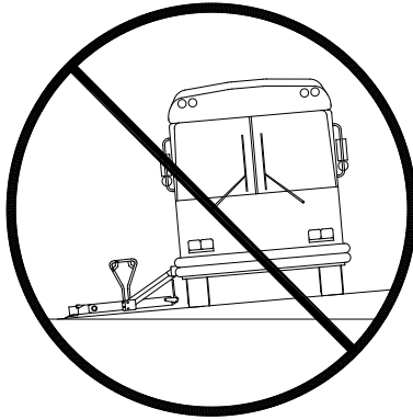
FIGURE 2-1: VEHICLE INCLINED DUE TO SLOPE
