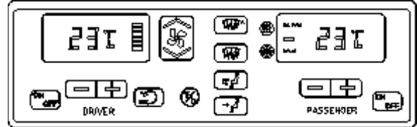
FIGURE 5: CENTRAL HVAC SYSTEM CONTROL UNIT 22296
