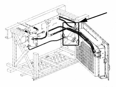
FIGURE 2 : ACTUAL FILTER DRYER TO REPLACE WITH PRÉVOST #453595
