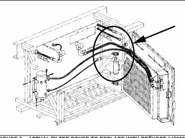
FIGURE 3 : ACTUAL FILTER DRYER TO REPLACE WITH PRÉVOST #453596
