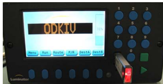
Figure 2-1. Flashdrive Inserted in ODK4
