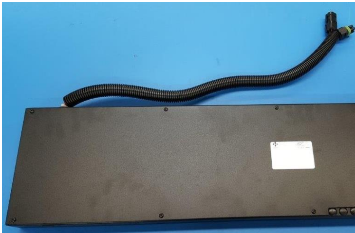
Figure 7A Power/communications and daisy-chain leads provided with the display are contained in a single sleeve
