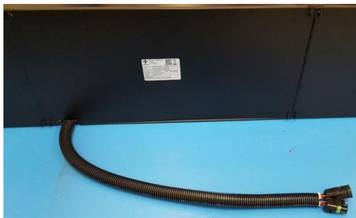
Figure 6A Power/communications and daisy-chain leads provided with the display are contained in a single sleeve
