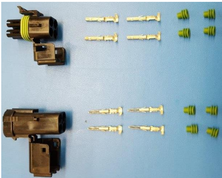
Figure 7B Power/communications and daisy-chain connectors: seals, crimps and housing
