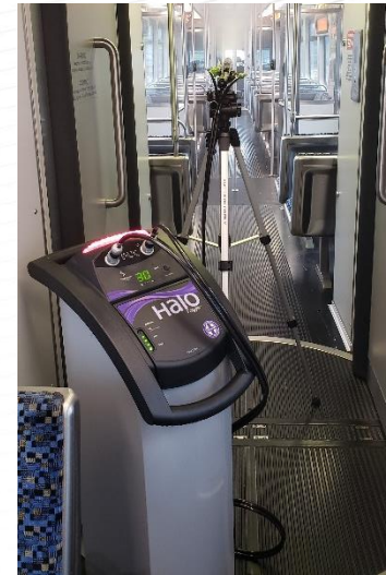
Dallas Area Rapid Transit (DART) using an EPA-approved fogging technology to disinfect a Light Rail Vehicle.
