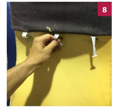
8 Remove the pull tabs out of the holes on the front side of the foam cushion.
