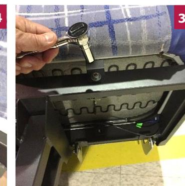
35 Reattach nut and washer to replace seat cushion with 1/2" socket wrench.
