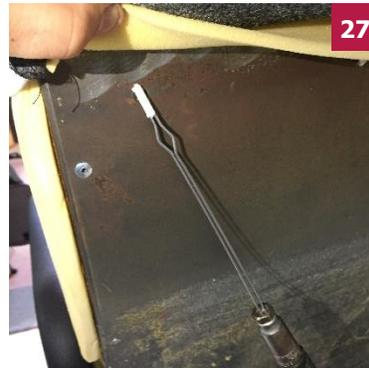
27 Push in the foam on the front and retract the pull tab through the steel back panel hole and rotate 90°. Repeat for all three pull tabs.
