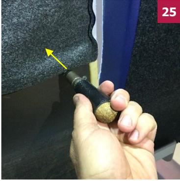
25 Insert a Pull Tab Tool through each opening in the back one at a time.
