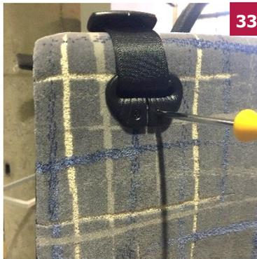
33 Replace belt guide screws with cross recess (Phillips) screwdriver.
