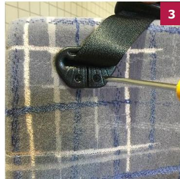
3 Remove two cross recess (Phillips) screws from the belt guide on the back cushion.
