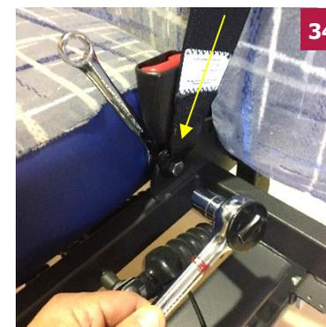
34 Reattached the belt end to the seat structure with a 5/8" socket wrench and 5/8" open end wrench.
