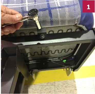
1 Remove nut and washer to remove seat cushion with 1/2" drive socket wrench.
