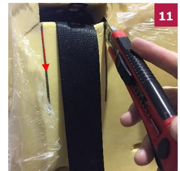
11 Cut through the foam down the lines with a sharp, (snap blade-retractable) utility knife.
