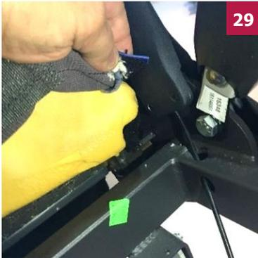
29 Pull the upholstery down the rest of the way and reattach **Velcro**® tabs at each corner.
