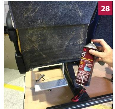
28 Pull the upholstery down to the armrest level and add spray glue on the lower portion of the back panel.
