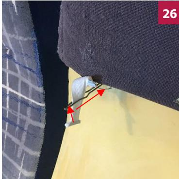
26 Retract the pull tab through each opening with the pull tab end in a horizontal orientation at the end of the tool.
