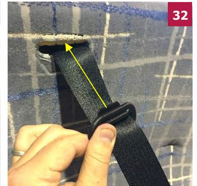
32 Reinsert the belt guide into the upholstery opening so that the upper tab is behind the upholstery.
