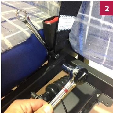
2 Remove belt end from the seat structure with a 5/8" socket wrench and 5/8" open end wrench.
