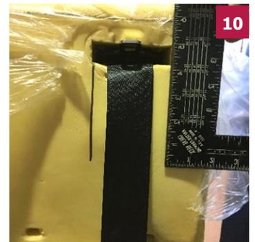
10 Mark two, 4" vertical lines from the bottom sides of belt openings in the foam.
