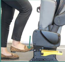
2. Use the small forward lock pedal to unlock seat from the current position
