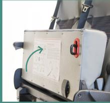
3. Push either the forward or rear foot pedal to slide seat in desired direction
