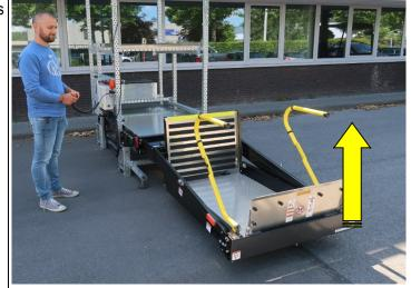
12 Unlock the handrails at the left and right side of the platform.
