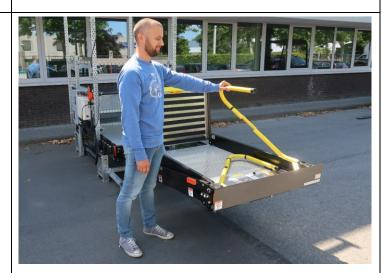
Fold the bridge plate back on top of the safety handrails.
