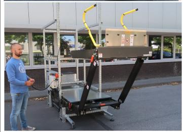
10 Repeat step 8 to disembark the vehicle and to lower the lift to ground level.
