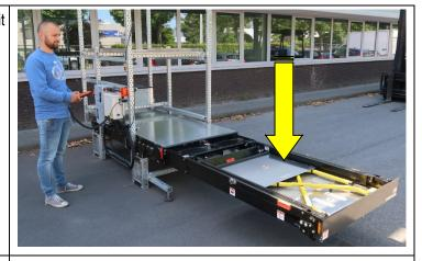
Press the STOW-button to stow the platform in its travel position inside the cassette. STOW fully until the lift frame is locked by the automatic cassette lock.
