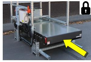
Switch OFF the electrical power to the lift by means of the cabin switch.
