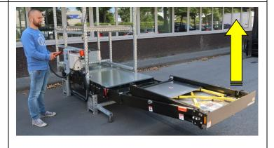
6 Manually open the bridge plate at the inboard platform edge.
