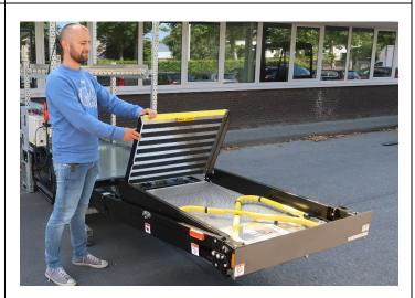
Press the DOWN-button to lower the platform until it stops automatically at the level of the cassette.
